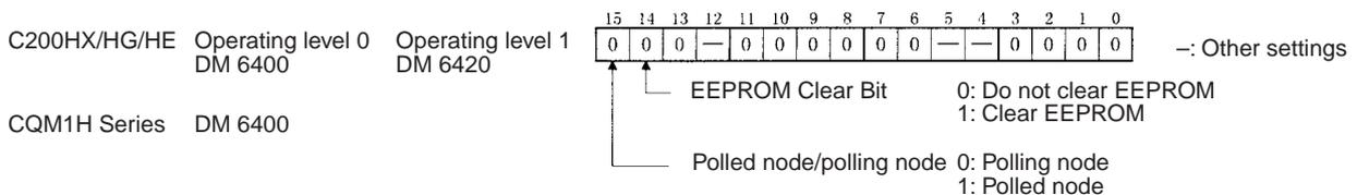
Check the above if the Controller Link Support Software can be used.
