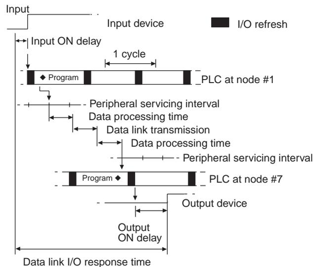
In this case, the data processing time required for data exchange and the data transmission time are not negligible and need to be included in the calculation. Each time can be determined as follows.
