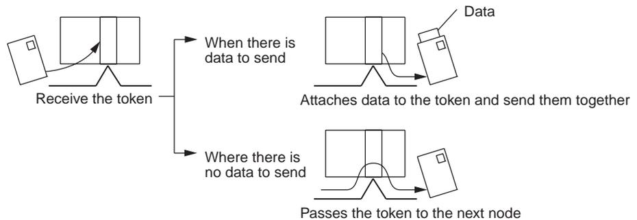
A token can be thought of as a circulating envelope. This envelope is circulated through the network and the person who receives the envelope will put a destination and a memo into the envelope to send his or her message to somebody else. This method is called “token passing.” The Controller Link Network is a bus network that uses token passing.
