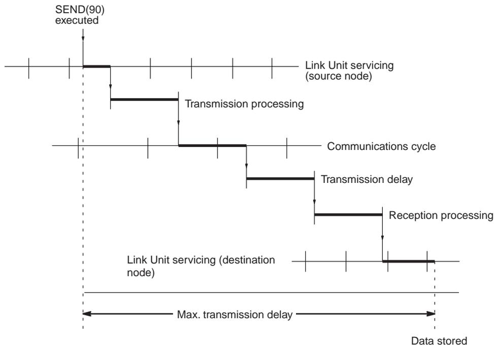
Max. transmission delay = Link Unit servicing interval (source node) + Transmission processing + Communications cycle time + Transmission delay + Reception processing + Link Unit servicing interval (destination node).
