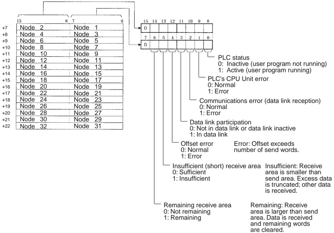
When the first data link status word is set to the default (0000) for either the manually set data link tables or automatically set data link tables (In the first data link status word parameter), the data link status is stored in the above area (CIO 1500 + 25 × (Unit No.) (+ 7 to +22)).
