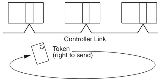
In a Controller Link Network, token passing is used to control network access. The right to send, called a “token,” circulates around the network. A node that receives the token is allowed to send data. If the node has data to send, it will attach the data to the token and send them together. If the node has no data to send, it will pass the token to the next node.
