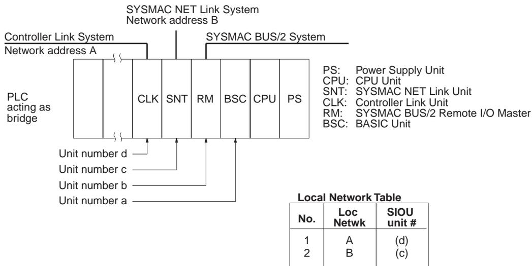
Do not register SYSMAC BUS/2 Master Units and BASIC Units in local network tables because these Units do not connect to networks.
