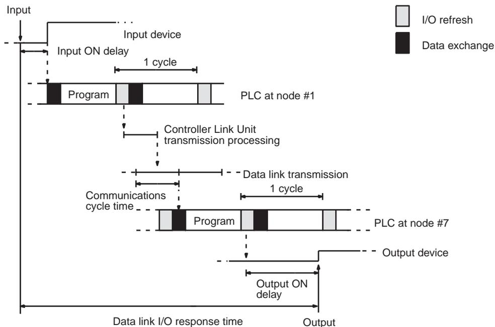
The equation for minimum data link I/O response time is as follows:
