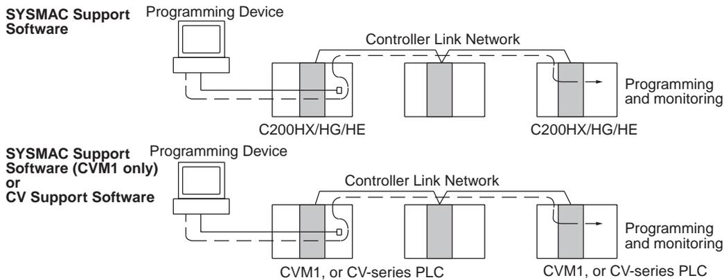
**Note** A factory automation node computer cannot remotely program or monitor. The node can only monitor Controller Link Network status.
