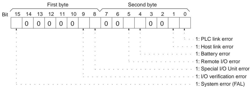
**FAL/FALS No. (response):** The number of the highest priority FAL/FALS error is returned as BCD between 00 and 99 (decimal) to the second byte. The first byte is always 00 (Hex). If no error has occurred, 0000 (Hex) is returned.
