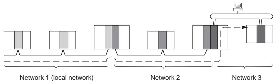
Although 2,012 bytes of data (including the header) can be sent and received with a Controller Link, the maximum amount of data is limited by any network the data passes through, i.e., the network with the smallest capacity will determine the limit.
