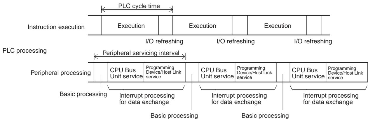
More than one data exchange can be executed during a PLC cycle, depending on the data exchange timing. If interrupt processing for data exchange is executed, the peripheral servicing interval will be lengthened by the time required for the interrupt processing (see 8-3-2 Data Processing Time on page 200).
