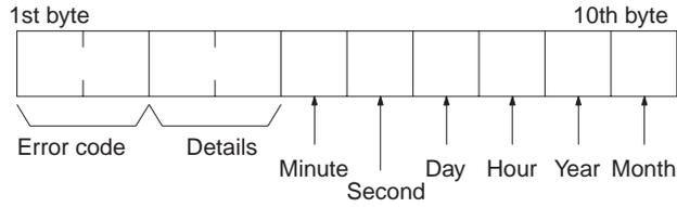
**Error code, details:** These parameters show the contents of errors. For details, refer to 9-3-2 *Error Codes*.
