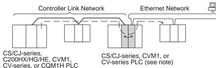
**Note** A data and communications protocol gateway is created between a Controller Link Unit and an Ethernet, SYSMAC NET, or SYSMAC LINK Unit mounted to the same CS/CJ-series, CVM1, or CV-series PLC.
