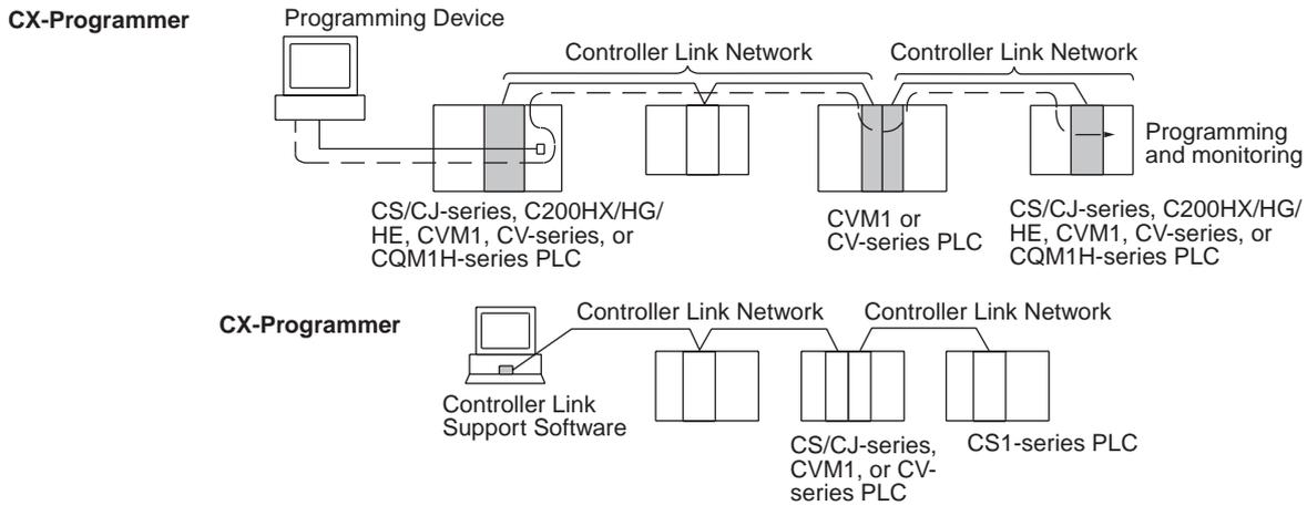
**Note** Remote programming and monitoring is possible from computer nodes.
