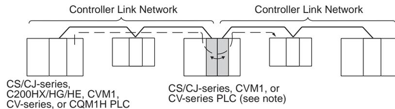
**Note** A data bridge is created between Controller Link Units mounted on the same CS/CJ-series, CVM1, or CV-series PLC.
