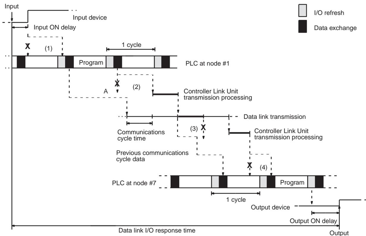
There are four points shown in the diagram above where processing is delayed, increasing the data link I/O response time.
