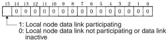
**Note** Data link status is valid only when the local node is participating in the data link. Confirm that the Local Data Link Active Bit is ON before referencing the data link status.
