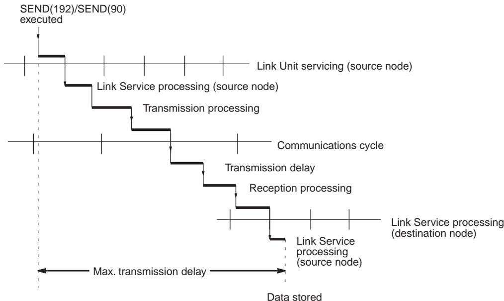
Max. transmission delay = Link Unit servicing interval (source node) + Link service processing (source node) + Transmission processing + Communications cycle time + Transmission delay + Reception processing + Link Unit servicing interval (destination node) + Link service processing (destination node)
