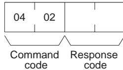
The DATA LINK STOP command can be received only while the data links are active. An error will occur if this command is sent at any other time.
