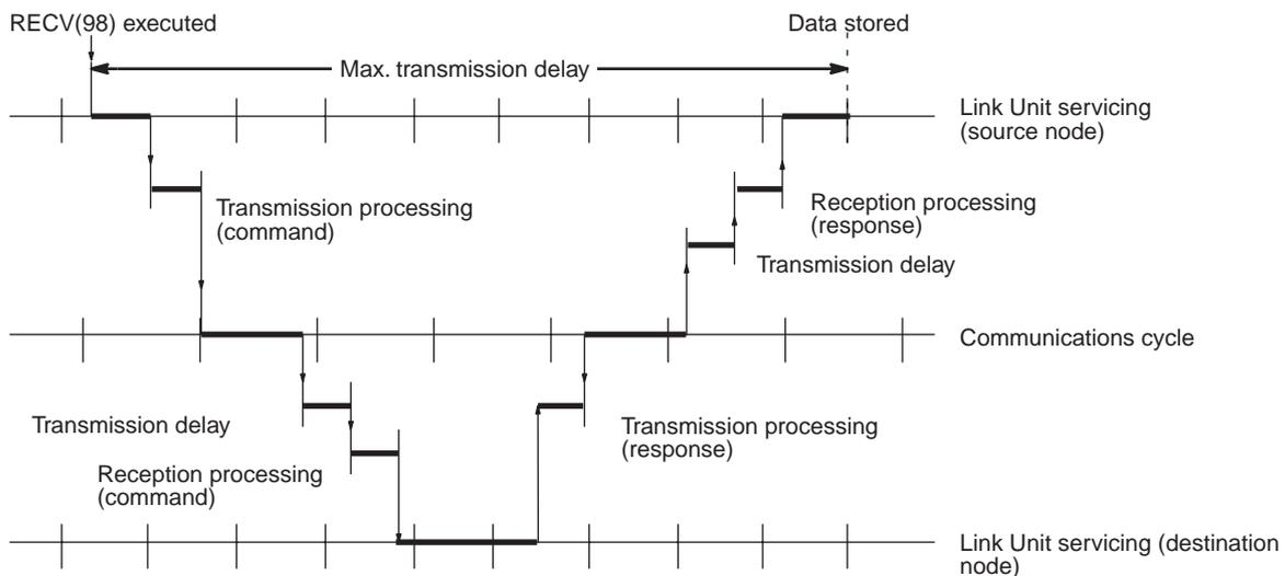
Max. transmission delay = Link Unit servicing interval (source node) + Transmission processing (command) + Communications cycle + Transmission delay (command) + Reception processing (command) + Link Unit servicing interval (destination node) + Transmission processing (response) + Communications cycle + Transmission delay (response) + Reception processing (response) + Link Unit servicing interval (source node).
