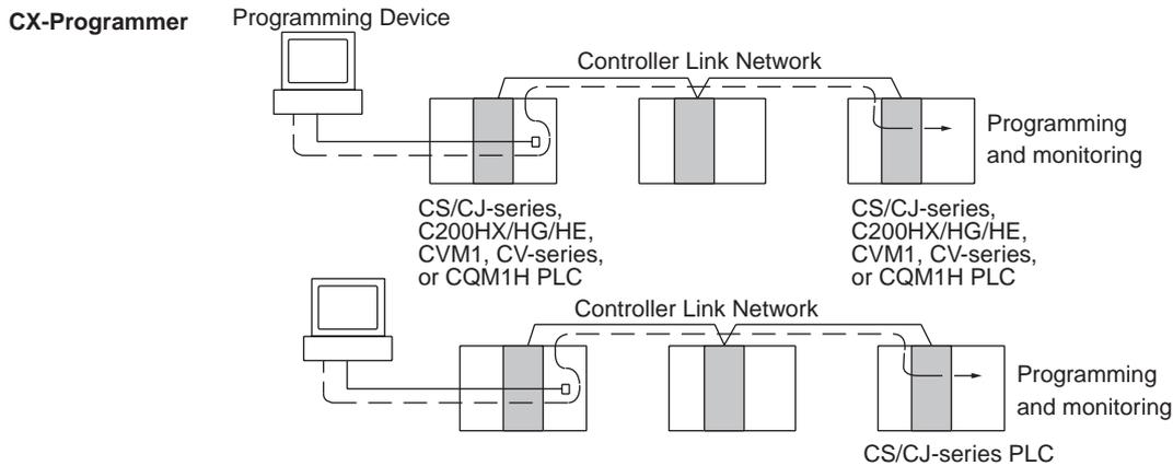
**Note** Remote programming and monitoring are possible from a factory automation node computer using the CX-Programmer.
