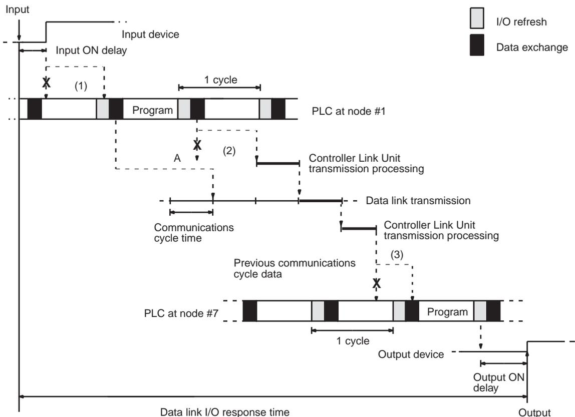
There are three points shown in the diagram above where processing is delayed, increasing the data link I/O response time.
