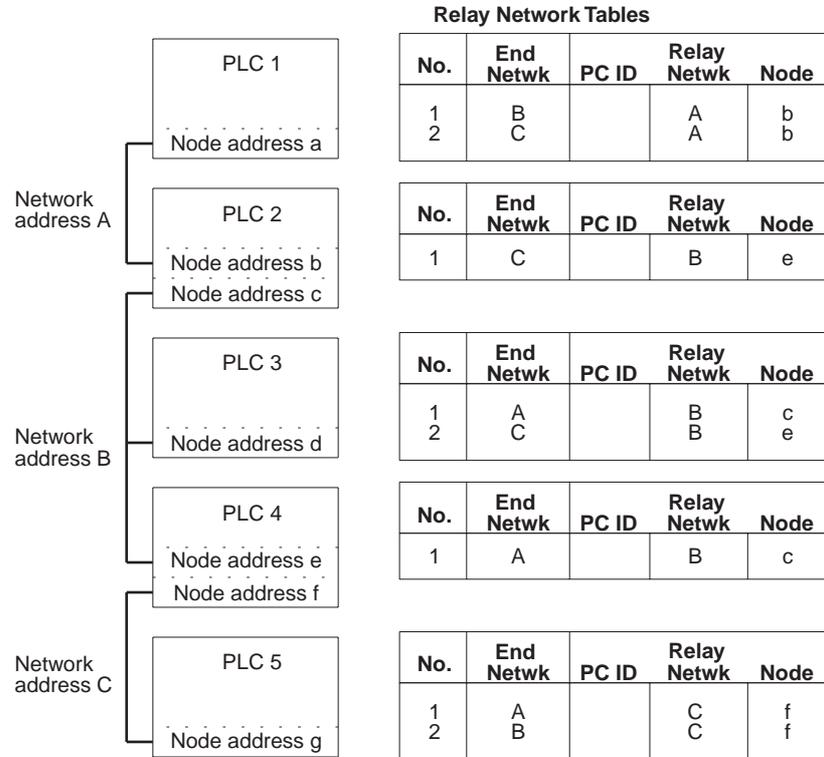
On closer examination of the relay network table for PLC#, we see that the relay network is B and the relay node is c when network A is the destination, and that the relay network is B and the relay node is e when network C is the destination.
