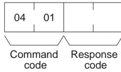
The DATA LINK START command can be received for either automatically or manually set data links. An error will occur if manually set data links are specified and yet data link tables do not exist.
