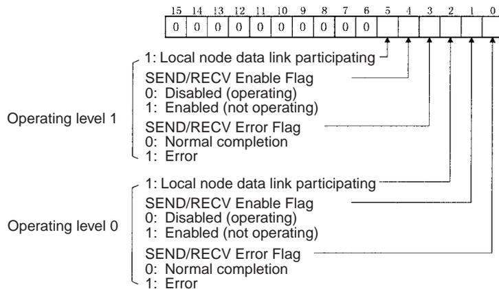
**Note** Data link status is valid only when the local node is participating in the data link. Confirm that the local node's data links are active in the operating level status in SR 252 before referencing the data link status.
