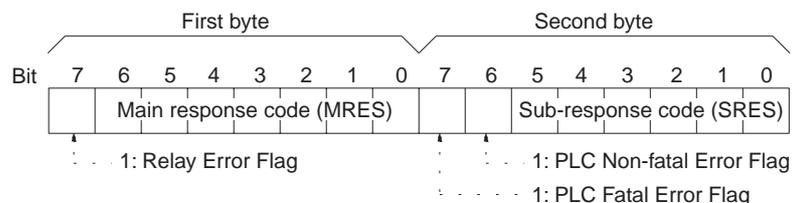
The main response code (MRES) in the first byte classifies the response and the sub-response code (SRES) in the second byte indicates details under the MRES classification.
