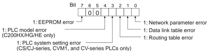
A network parameter error, data link table error, or routing table error occurs if an error is discovered when the parameters and tables are checked at power up.
