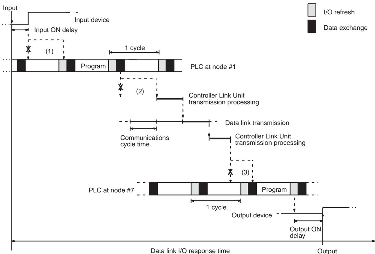
There are three points shown in the diagram above where processing is delayed, increasing the data link I/O response time.
