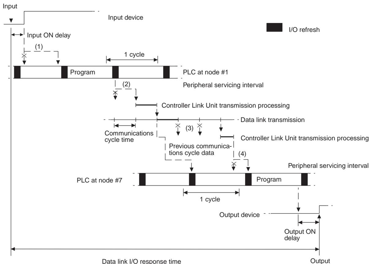
There are five points shown in the diagram above where processing is delayed, increasing the data link I/O response time.
