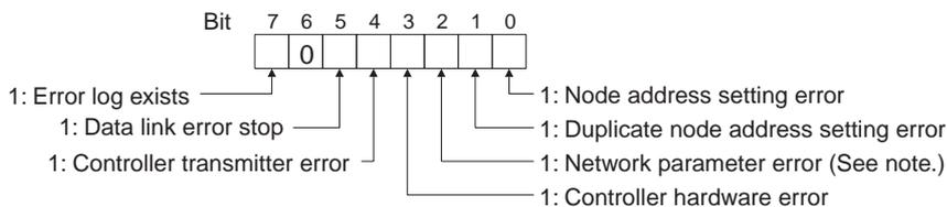
**Note** With CS/CJ-series Optical Controller Link Units, this bit will be 1, even if the Unit is mistakenly connected to an Optical SYSMAC LINK Network.
