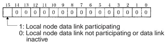
**Note** Data link status is valid only when the local node is participating in the data link. Confirm that the Local Data Link Active Bit is ON before referencing the data link status.
