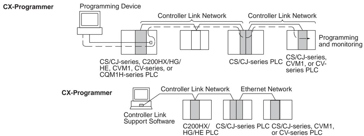
**Note** Remote programming and monitoring is possible from computer nodes.
