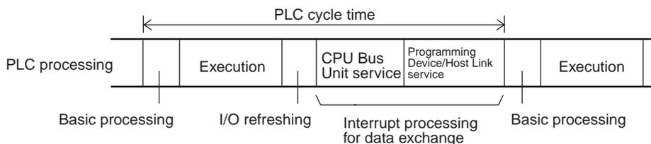
If interrupt processing for data exchange is executed, the PLC cycle time will be lengthened by the time required for the interrupt processing (see 8-3-2 Data Processing Time below).
