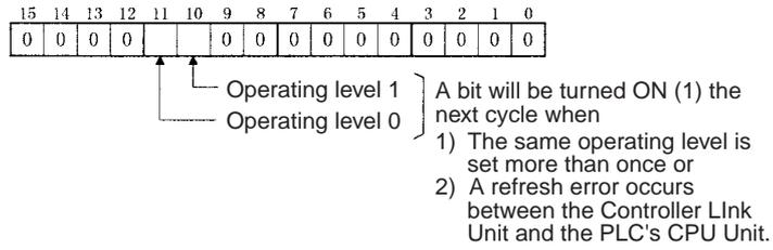
**Routing Table Error/Unit Restart Bits: AR 01**
