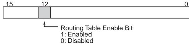
DM 6450 through DM 6499 can be used as desired if the Routing Table Enable Bit is set at 0 to disabled routing tables.
