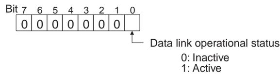
**Data link type (response):** Indicates the data transmission status of the local node's data links. It is configured as shown in the following diagram. This parameter is valid only during data link operation. While data link operation is inactive, the value from the previous operation is retained.
