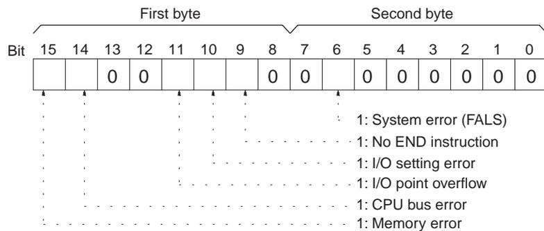
**Non-fatal error data (response):** The contents of non-fatal error information from the PLC. (For details refer to the operation manual of the PLC that is being used.)
