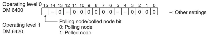
**CVM1 and CV-series Controller Link Units**
