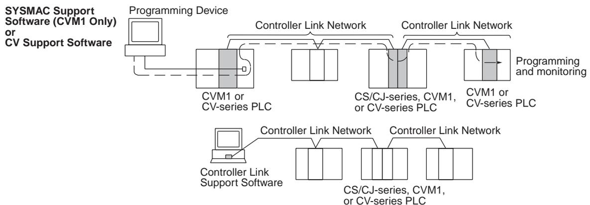
**Note** Remote programming and monitoring is not possible from computer nodes. Computer nodes can only monitor Controller Link Network status. A Programming Device connected to a C200HX/HG/HE PLC cannot remotely program or monitor a node on a remote network.
