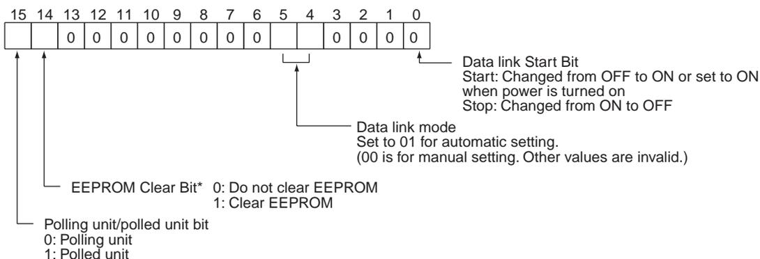
\*Clears the network parameters, data link tables, and routing tables stored in EEPROM in the PLC's CPU Unit.
