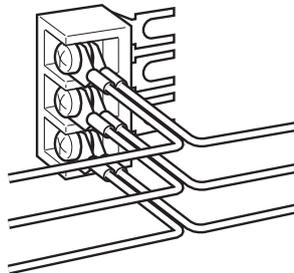
2. Remove the terminal block cover from the communications terminal block on the Controller Link Unit and loosen the three screws on the communications terminal block. (If adjacent Units are close enough to interfere with work, remove the three screws.)
